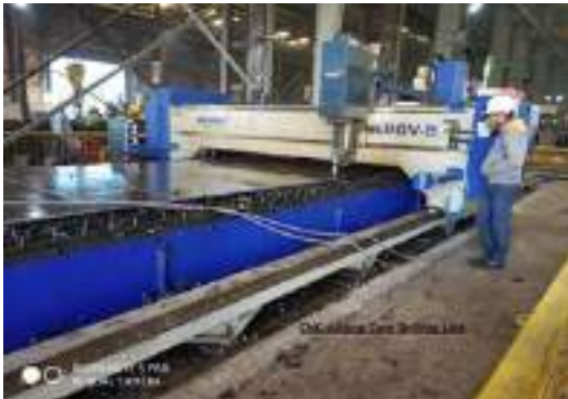
CNC Plamill Cutting Cum Drilling Line
